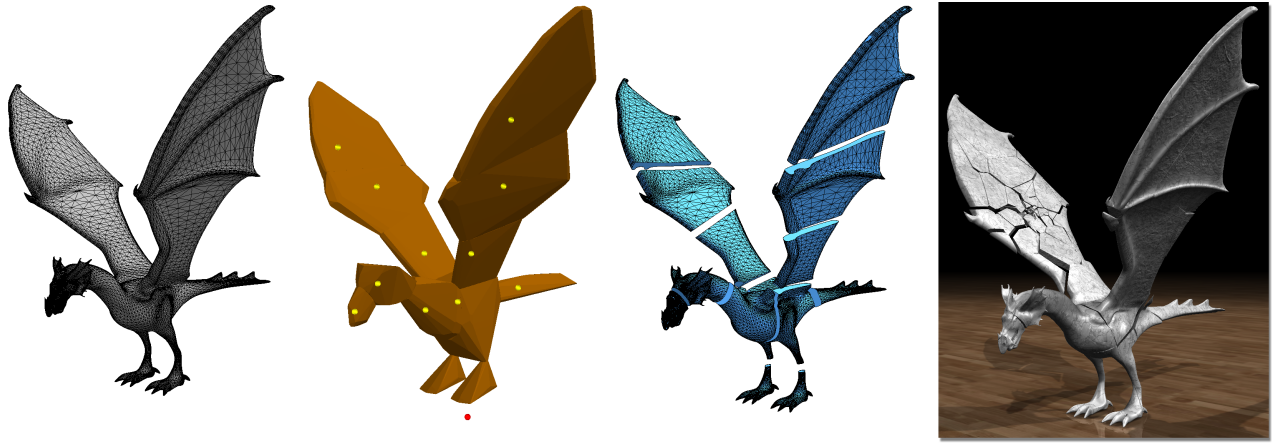
Figure 10: Volumetric Approximate Convex Decomposition of a dragon model with 40k vertices and 80k triangles. Placing twelve nodes intuitively in a matter of seconds results in a tight fitting decomposition that makes fracturing this high resolution mesh possible in real time. From left to right: Original model, compound mesh, one split mesh per convex (shrunk for visualization) and destruction of the model at runtime.
